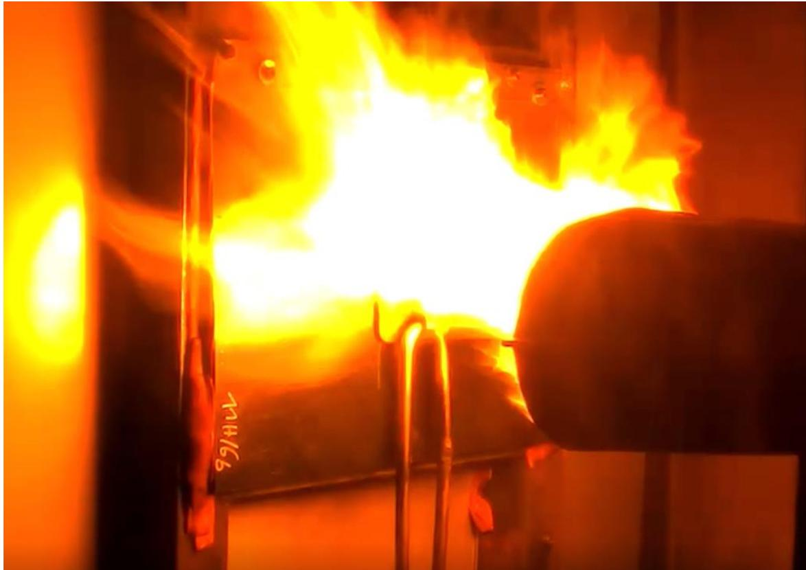
Picture shows a fire test of the 600x400mm thermoplastic composite panel and the bracket. Both the loading hook and the flame torch can be seen.
