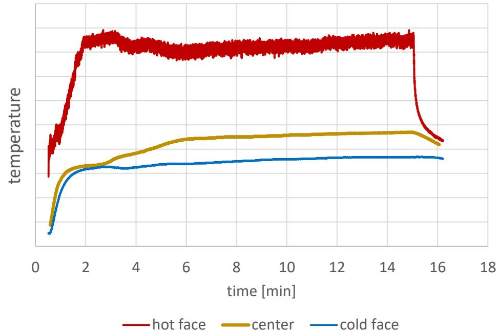
Graph shows the temperature profile of a point close to the center of the thermoplastic panel during a 15 minute long fire test. Data are from the hot burner face, the center layer of the panel measured by FBGS and the cold back face of the panel.
