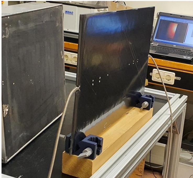
Picture shows an instrumented 400x300mm panel made of PAEK thermoplastic carbon fiber composite during calibration tests. The optical fiber egress has been protected with robust stainless steel corrugated tubing.
