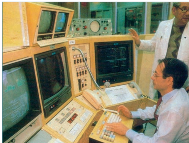
Typical brown color console for the centralized operation of Mark IV A, in a glass cubicle “the fishbowl” in the middle of the same room. ■
